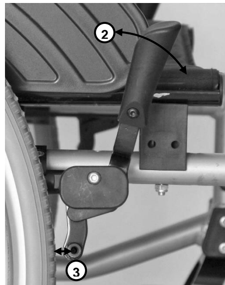
Brake disengaged (wheelchair rolls)
