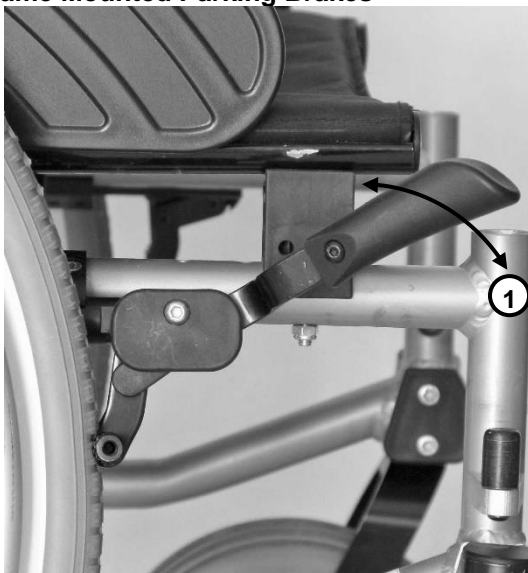
Brake engaged (wheelchair doesn't roll)
