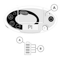
The battery gauge (A) shows the status of the installed battery charge level when the concentrator is turned on and when the concentrator is off but connected to an external power source. The number of illuminated segments (B) of the battery gauge (A) indicates the charge level of the installed battery. If two batteries are installed the indicated charge level is that of the least charged battery.
