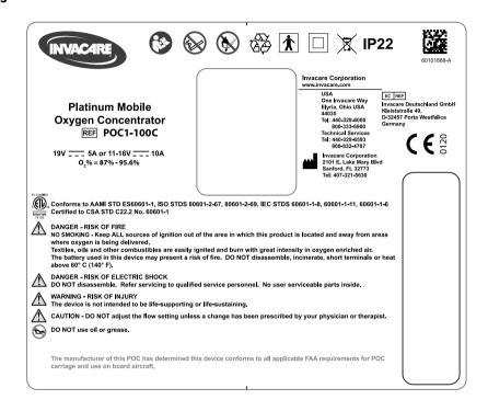
The label is located on the back of the concentrator. The serial number is located on the right side of labels shown here.
